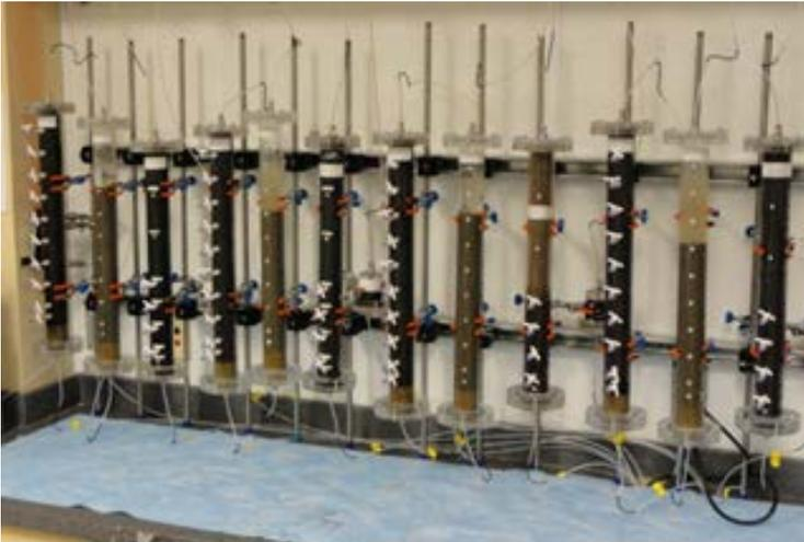
Geosyntec designed and managed a treatability column study and developed PRB design parameters.
